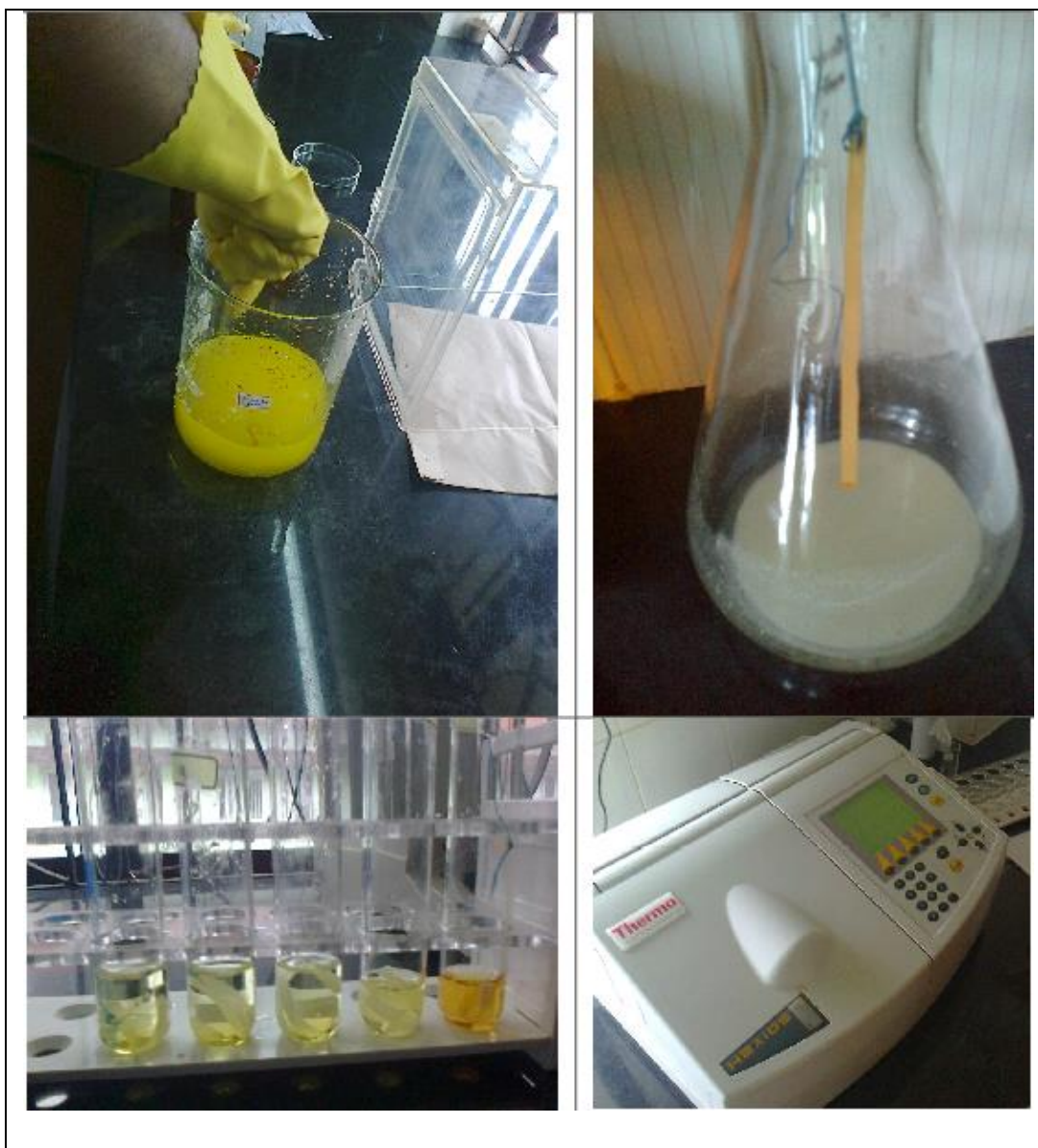
Plate 2. Evaluation of HCN content in powdery cassava sample
