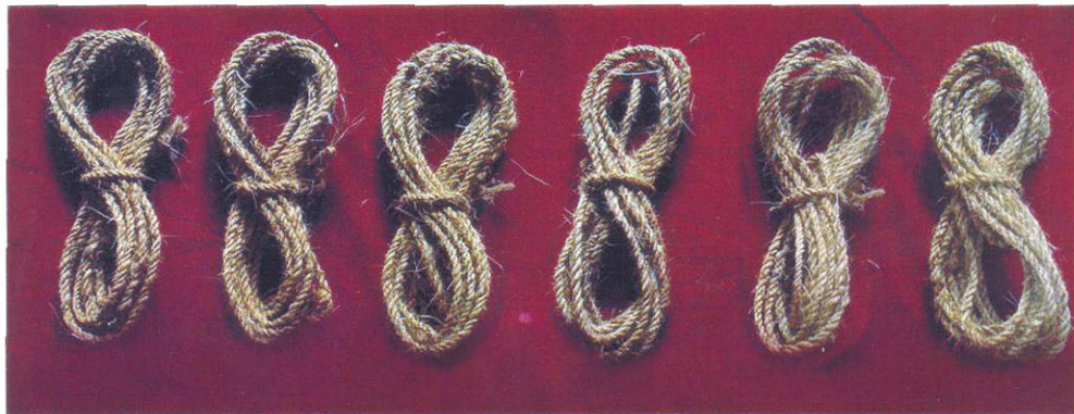
I II III IV V VI Coir yarn obtained from different damage categories
