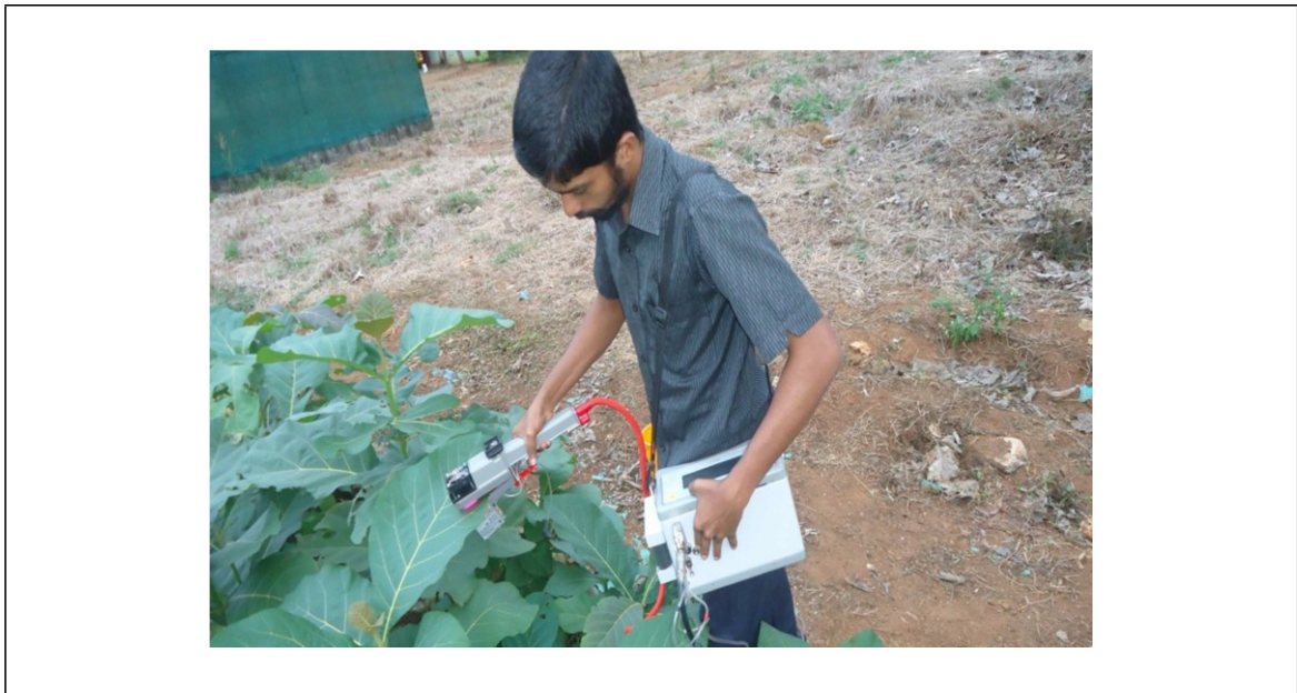
Plate 4. Estimation of photosynthetic rate and transpiration rate using IRGA
