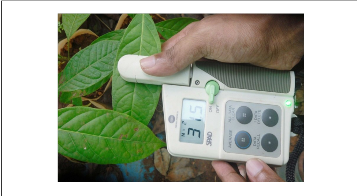
Plate 3. Estimation of chlorophyll content using SPAD meter
