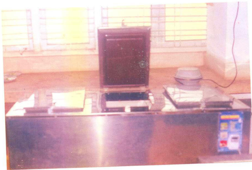
Plate 1. Top loading cooler used for chilling minimally processed tender coconut
