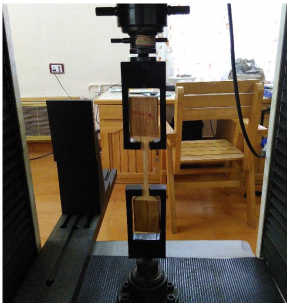
Plate 13. Test for tensile strength parallel to grain
