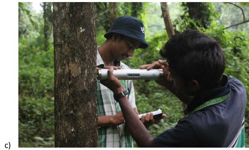
Plate 2. Pictures showing various field activities on standing trees, a) taking girth measurement of standing tree b) collecting core sample c) taking pilodyn penetration depth d) making tree-sonic timer reading and e) showing tree-sonic timer set up on standing trees.
