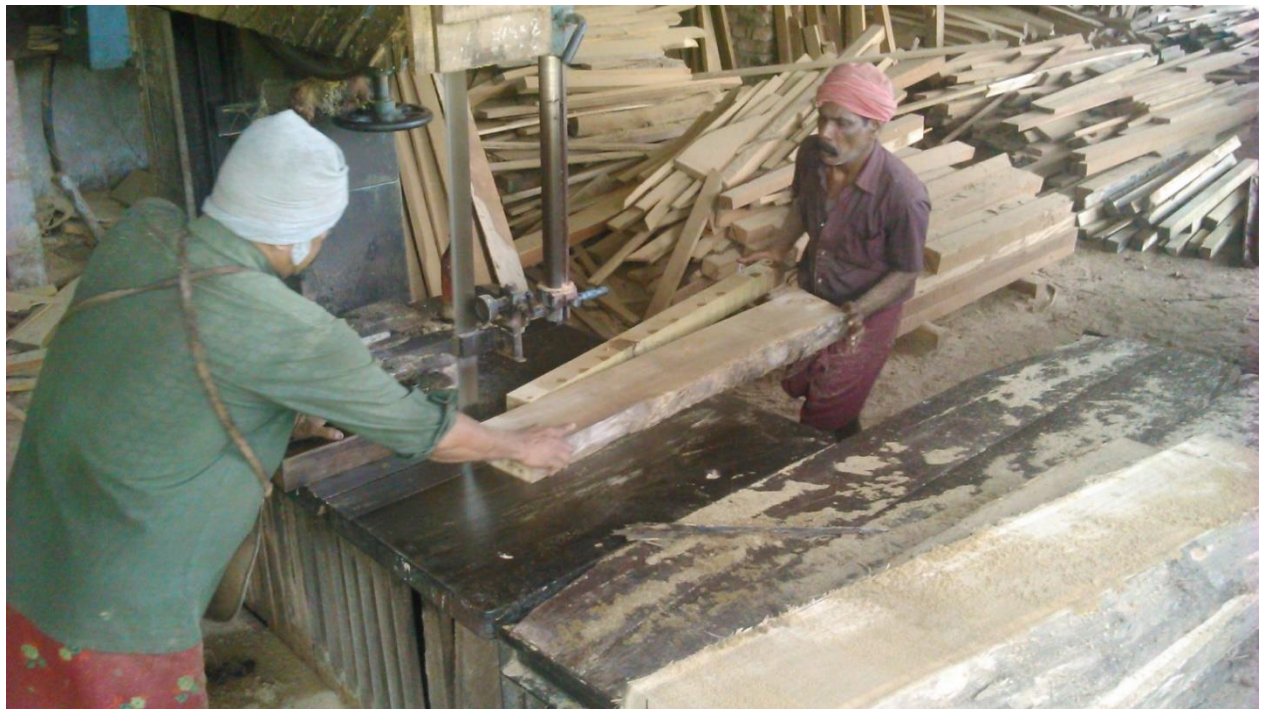
Plate 4. Sawing of logs using band saw (a) and further conversion using re-saw machine (b) to scantlings for conducting strength tests.
