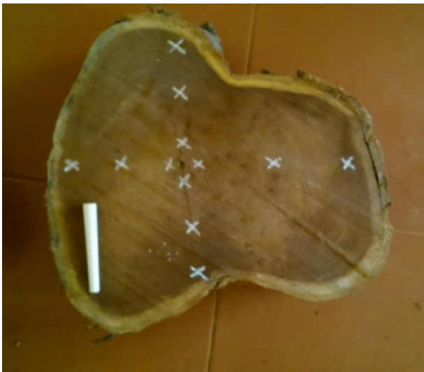
Plate 5. a) Collection of discs from logs for conducting NDT measurements b) Discs showing positions at which measurements were taken at the end cross section of logs and discs using Pilodyn. c) Making Pilodyn penetration depth readings on the discs.
