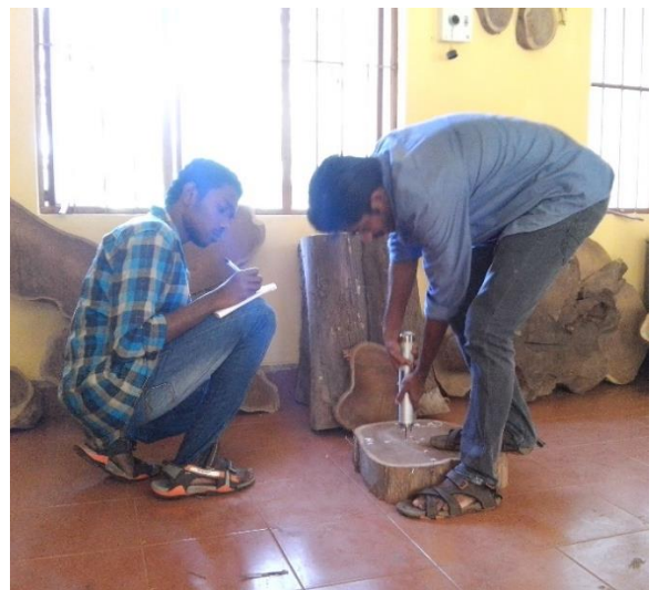
Plate 5. a) Collection of discs from logs for conducting NDT measurements b) Discs showing positions at which measurements were taken at the end cross section of logs and discs using Pilodyn. c) Making Pilodyn penetration depth readings on the discs.
