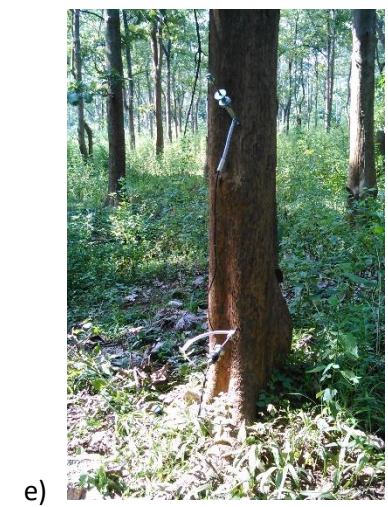
Plate 2. Pictures showing various field activities on standing trees, a) taking girth measurement of standing tree b) collecting core sample c) taking pilodyn penetration depth d) making tree-sonic timer reading and e) showing tree-sonic timer set up on standing trees.
