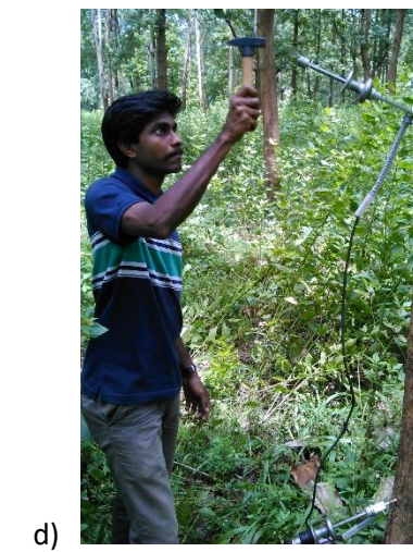
Plate 2. Pictures showing various field activities on standing trees, a) taking girth measurement of standing tree b) collecting core sample c) taking pilodyn penetration depth d) making tree-sonic timer reading and e) showing tree-sonic timer set up on standing trees.
