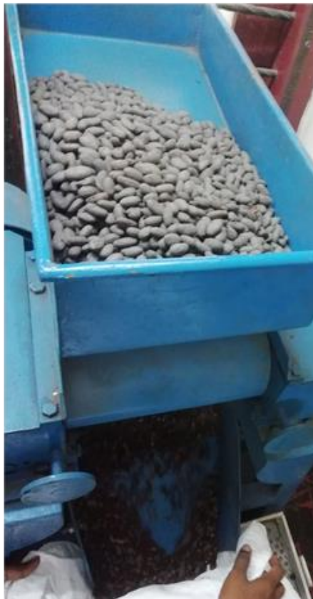
Plate 13. Dehusking (Knibbling) of roasted cocoa beans
