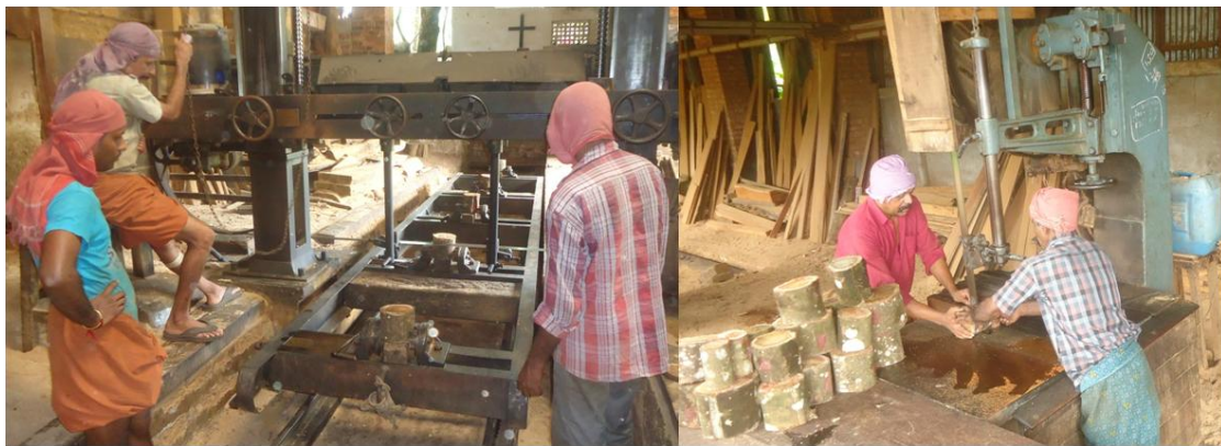
Plate 8. Further conversion of billets and discs into standard sample size in saw mill
