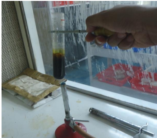
Figure 12. Maceration of slivers using Jeffrey's method.
