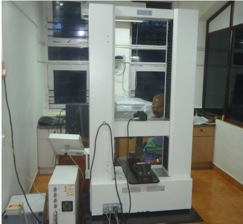
Plate 14. 50 kN capacity Universal Testing Machine (Shimadzu, Japan).
