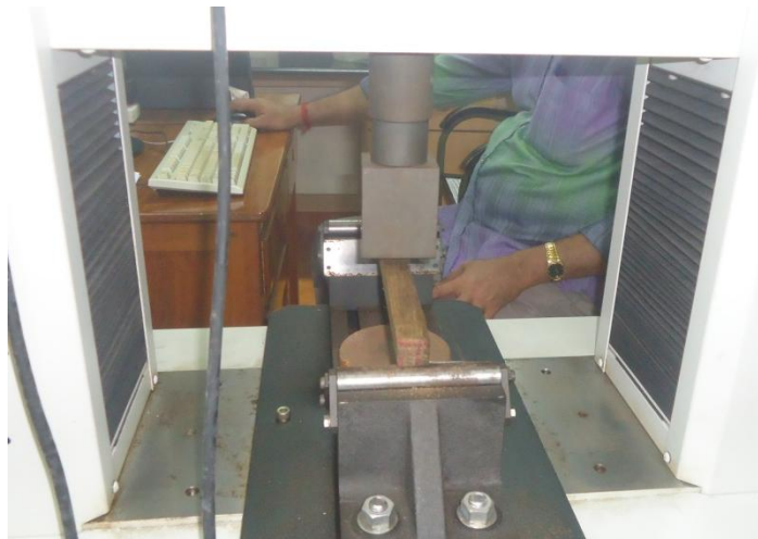
Plate 15. Sample loaded for testing the static bending strength.
