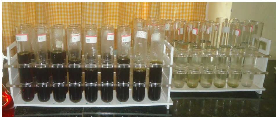
Plate 13. Allowing the macerated fiber to settle down. The test tubes with clear solution are ready for extraction of fiber.
