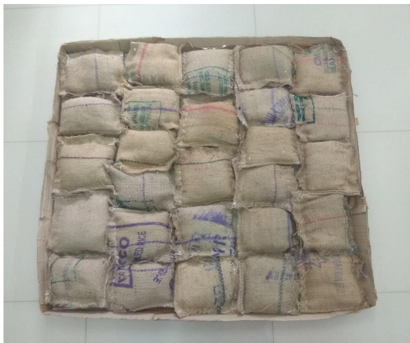
Plate 4. Jute bags containing 1 kg of rice arranged in a single layer in 1 m 2 for pesticide residue analysis
