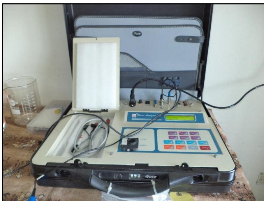
Plate 3.1 Systronic water quality analyser
