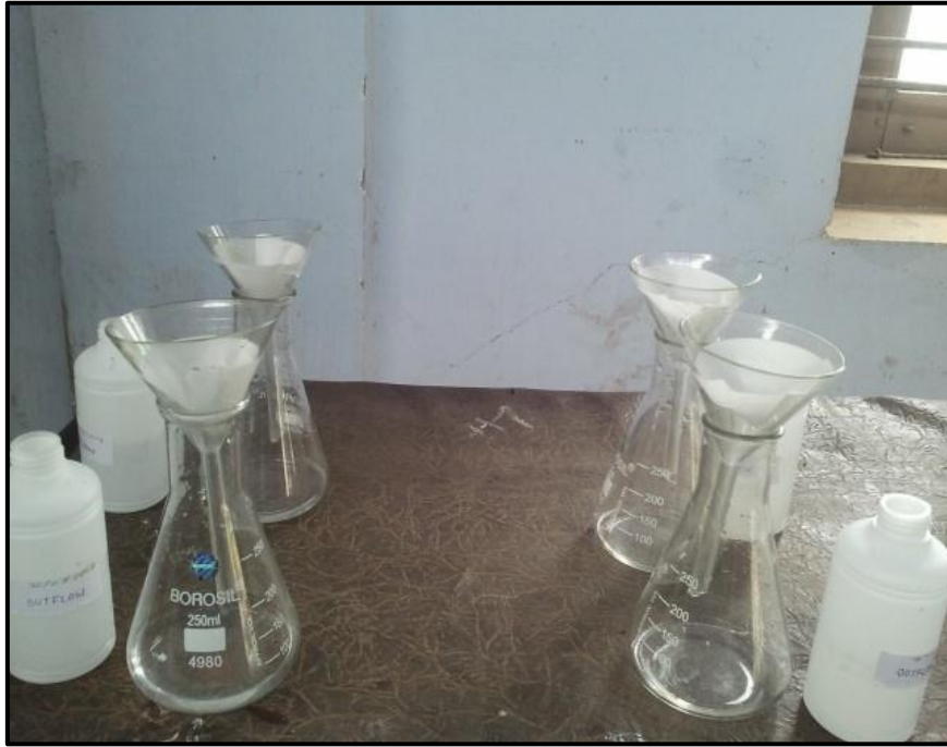
Plate 3.4 Gravimetric experimental setup for total suspended solids
