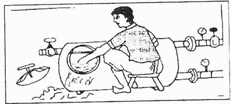
Fig. 7.2. Replacement of sand in sand filter
