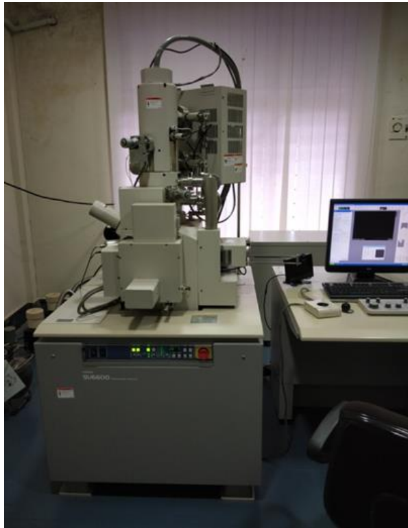
Plate 3.14 Hitachi SU6600 Variable Pressure Field Emission Scanning Electron Microscope (FESEM)
