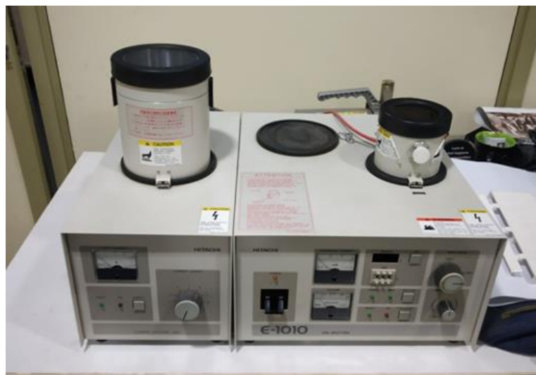
Plate 3.15 Ion sputter coating unit
