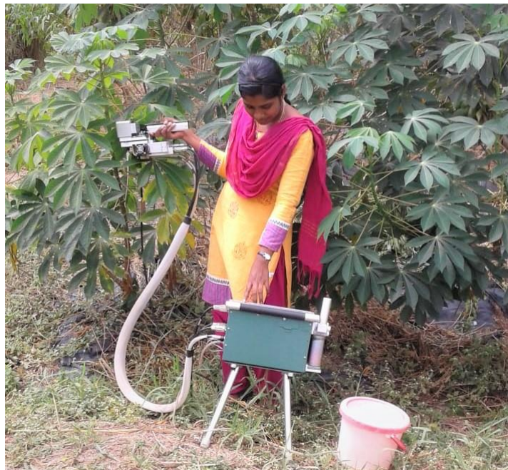
Plate 3.3: Recording photosynthetic parameters using LI6400 portable photosynthesis system in the field.
