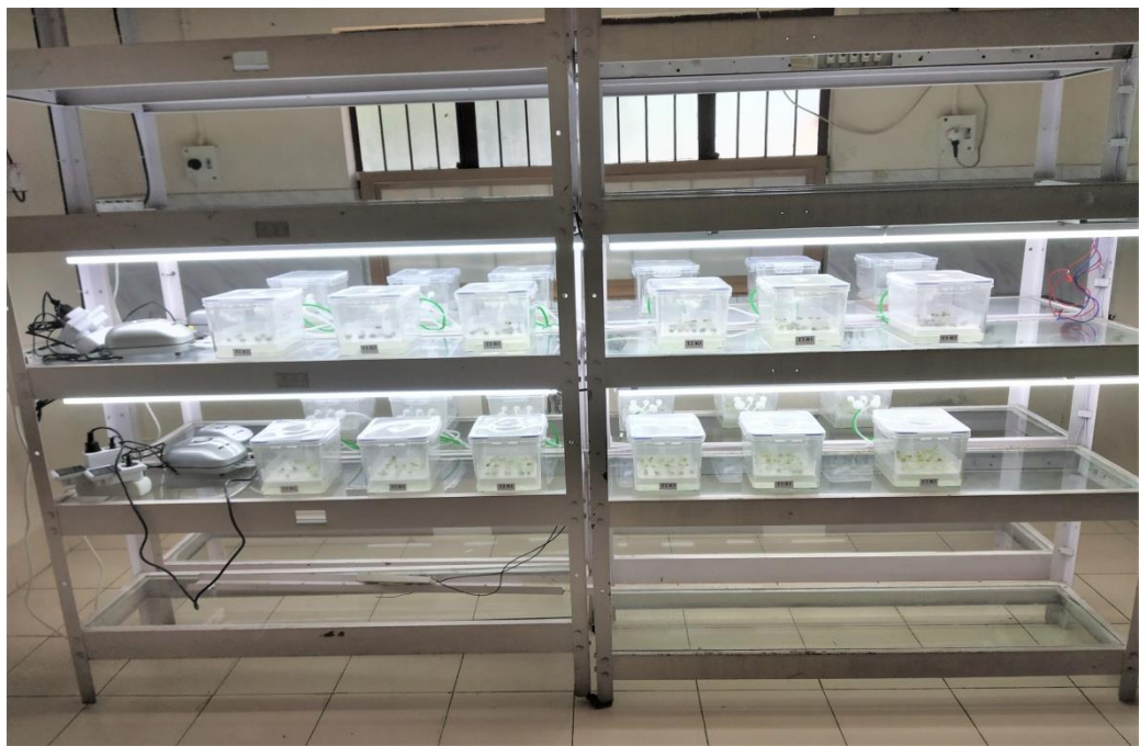
Plate 1. Experimental setup with Plantform temporary immersion bioreactor
