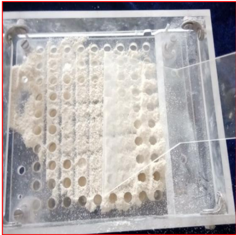
a. Spreading the filler material
