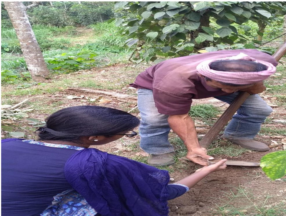
Plate. 2. Soil sample collection using core.
