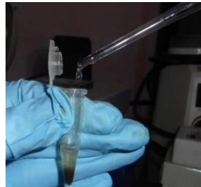
h. Glacial acetic acid added, centrifuged and sediment washed 5 times
