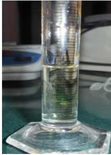
d. Acetolysis mixture freshly prepared (Acetic anhydride : Conc. Sulphuric acid, 9:1)
