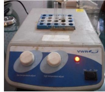
f. Heated for 10 min at 45 °C with intermittent stirring
