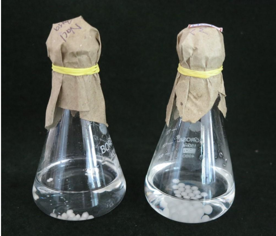
Plate 16. Encapsulated beads of PGPR mix-I amended with 10% Standard starch in sterile saline solution
