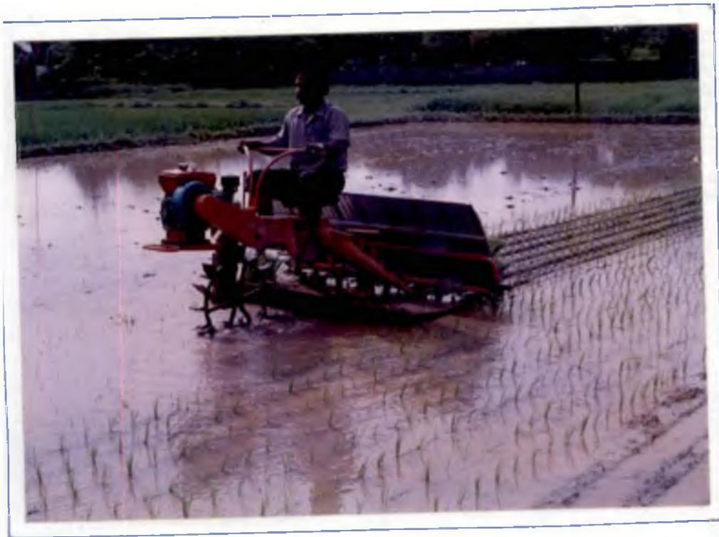
Plate III 8-row YANJI SHAKTHI Rice Transplanter in action
