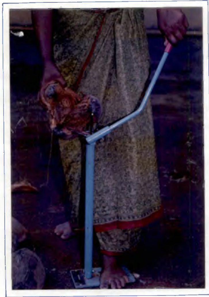
Plate V Coconut dehusking tool " Keramitra " designed by Kerala Agricultural University
