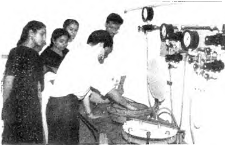
Demonstration with Pressure Plate Apparatus
