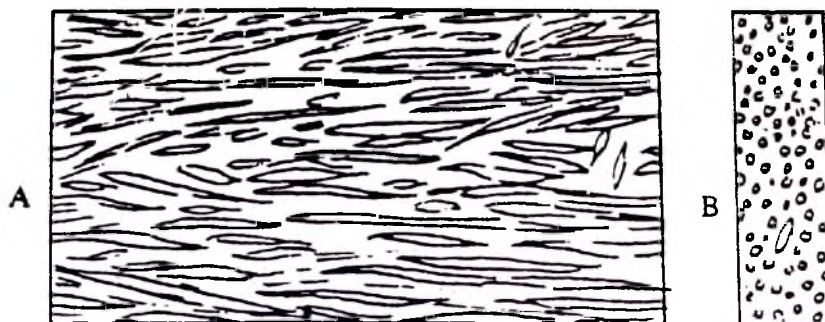
Very low density wood texture from the peripheral zone of stem apex. Note: High concentration of very thin fibre walled vascular bundles (nearly in gelatinous state).
