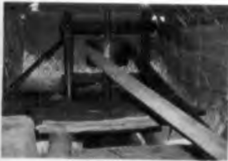
Petti and Para device for drainage in Kole paddy field
