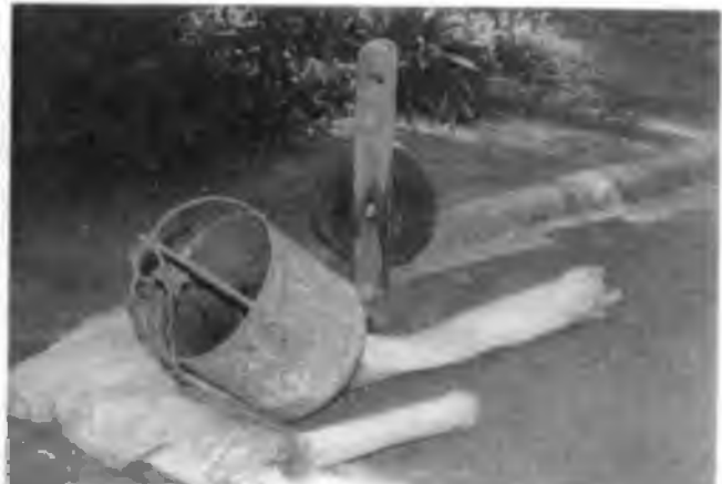
Self emptying rope and bucket lift ("Kaiathekku")
