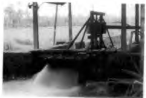
Petti and Para device for drainage in Kole paddy field
