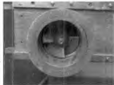
Figure 3.18 Close-up view of the impeller used in Petty and Para
