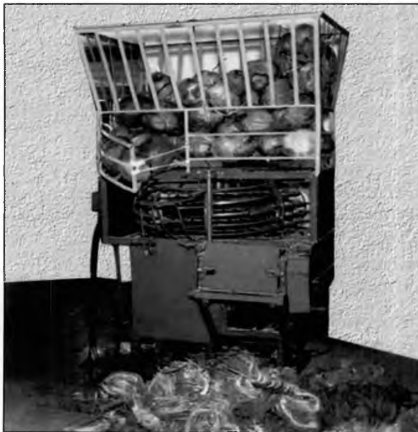
Plate 2.2 Power operated continuous coconut husking machine
