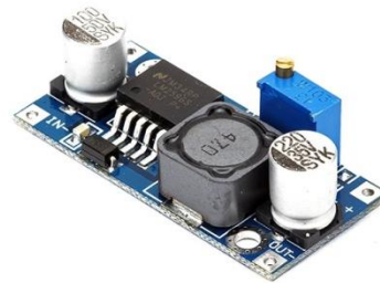
Fig. 4.12 LM2596 buck converter
