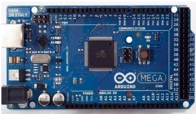
Fig. 4.8 Arduino Mega microcontroller board
