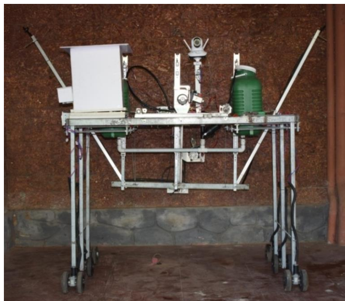
Fig. 4.23 Developed prototype of semi-autonomous robotic platform
