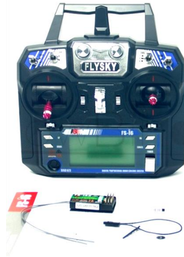
Fig. 4.10 Transmitter remote controller with receiver
