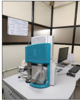
Plate 3.5. Scanning electron microscope instrument used for pollen studies (Tescan Vega 3 model)
