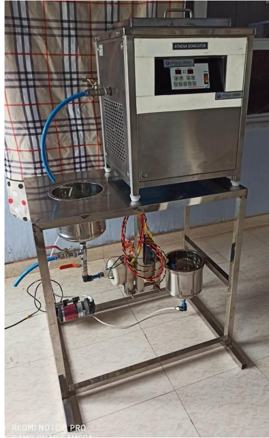
Figure 3.3 Developed Ultrasound assisted UV treatment system
