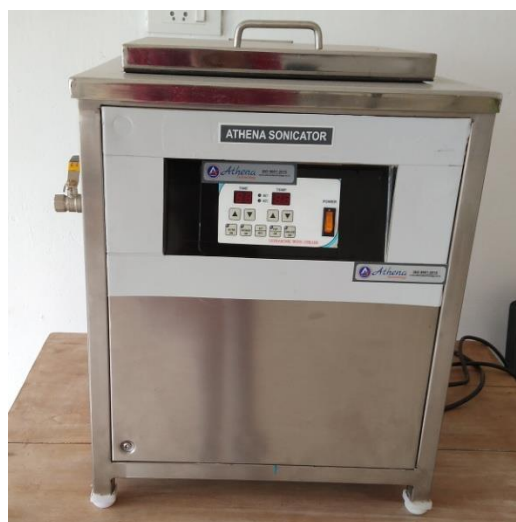
Figure 3.4 Ultrasonic bath with chiller
