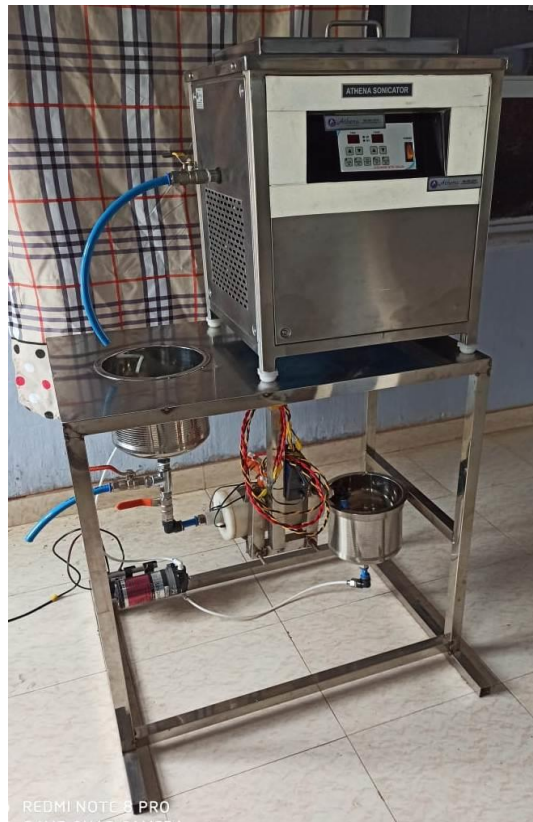
Figure 4.1 Developed Ultrasound assisted UV treatment system
