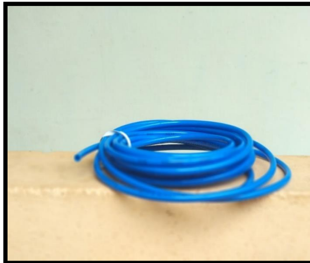
Figure 3.9 Pneumatic pipes/ tubes
