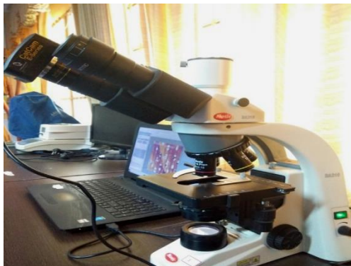
Catcam 500E microscope camera on a Motic BA210 trinocular microscope
