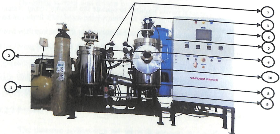
Plate 3.2. Developed Vacuum Frying System (KCAET, Tavanur, Kerala)
