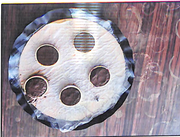
Plate 2. Saturated pressure plate and soil samples
