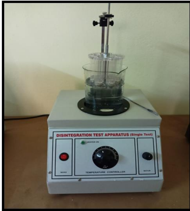
12a. Tablet disintegration test apparatus
