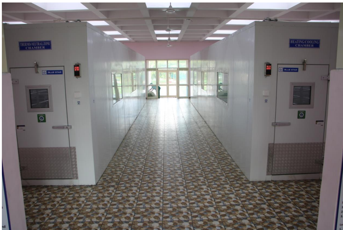
Plate 3.1: Climate chamber: Thermo-neutral Zone Chamber (left) and Heating/ Cooling Chamber (right) outside view
