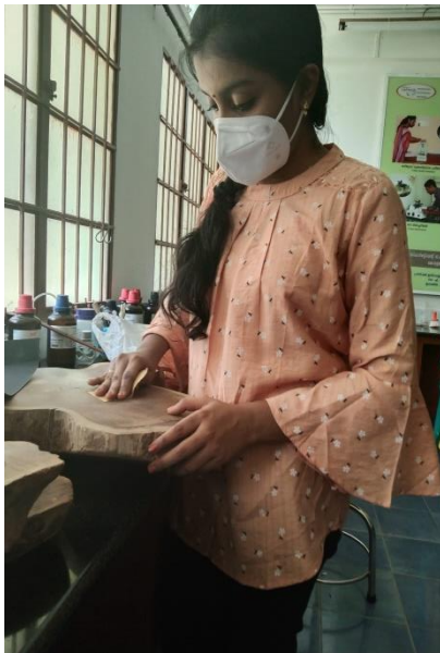
Figure 4: Smoothing of wooden discs surface using sandpaper
