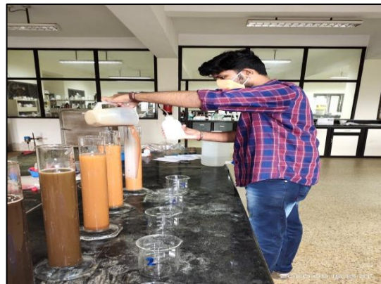
Plate 7. Soil texture analysis using Bouyoucous method.
