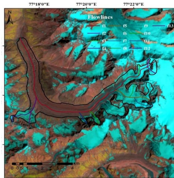
Figure 15. 13 flowlines are delineated for the glacier no. 305 including central flowline and tributary flowlines. Flowlines are digitized at 150m distance from the boundary. Each flowline is separated with 300-400 m.
