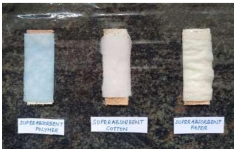
Plate 3: Materials used for the study : Super absorbent polymer, super absorbent cotton and super absorbent paper
