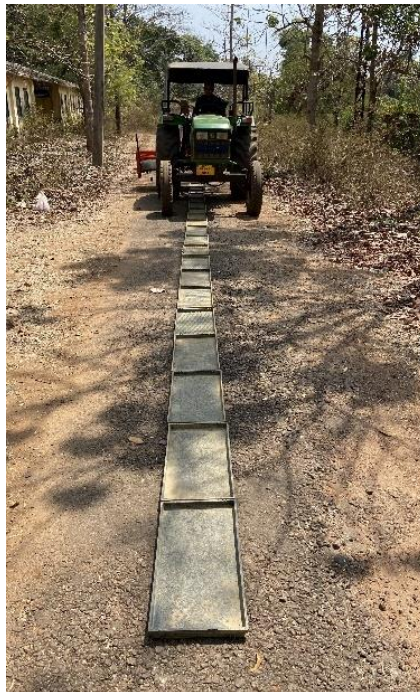
Plate. 3.18 Laboratory test for fertilizer distribution pattern
