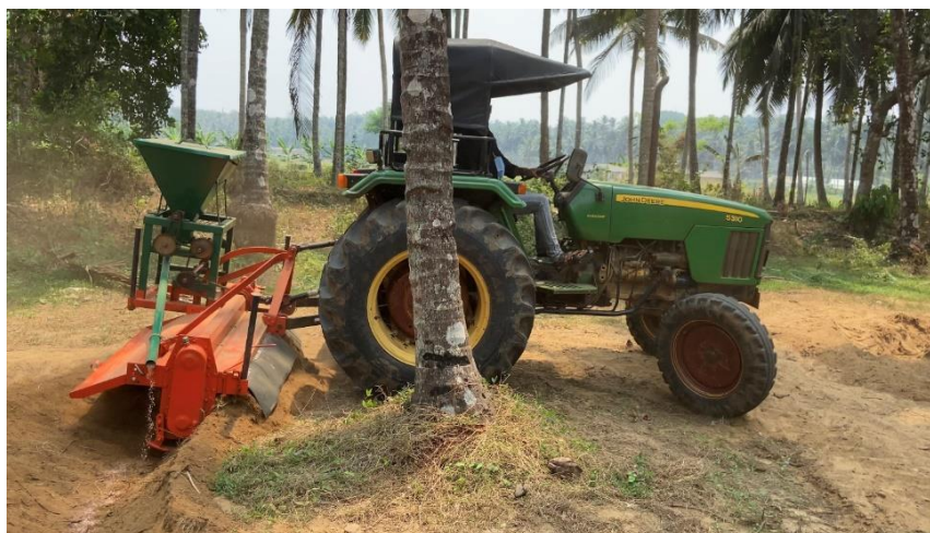
Plate. 3.20 Testing of tractor operated basin lister cum fertilizer applicator
