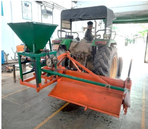
Plate. 3.19 Laboratory test for fertilizer application rate
