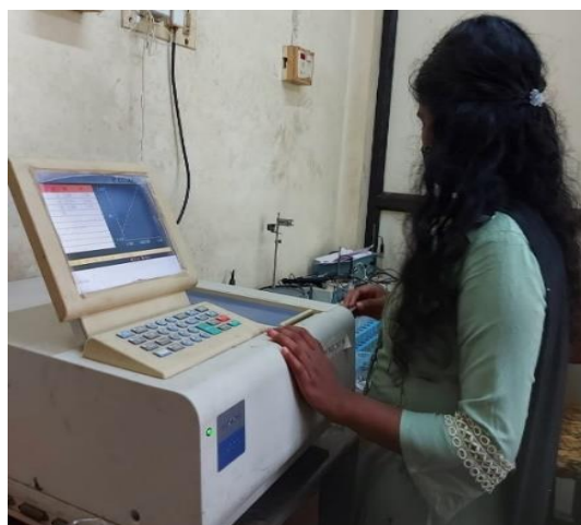
Plate 3.9 Determination of sulphur content using UV Spectrophotometer
