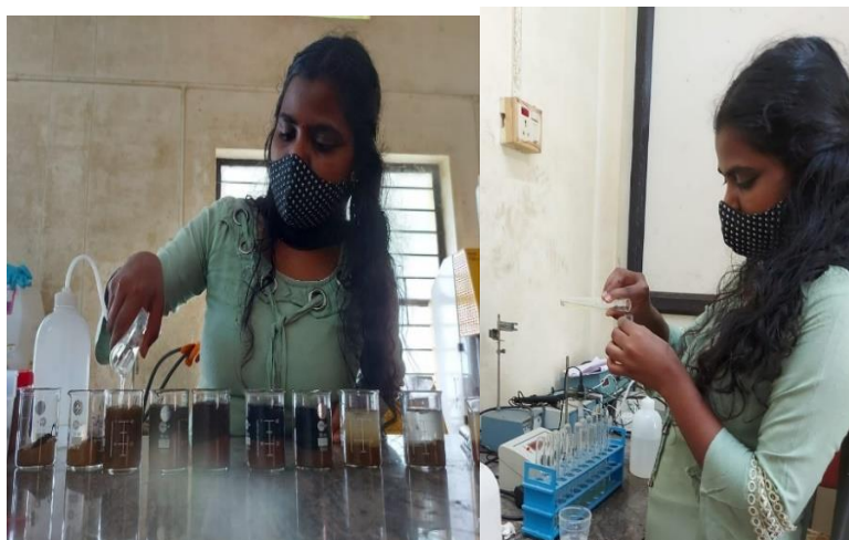
Plate 3.10 Determination of Boron content by using Hot water extraction method
