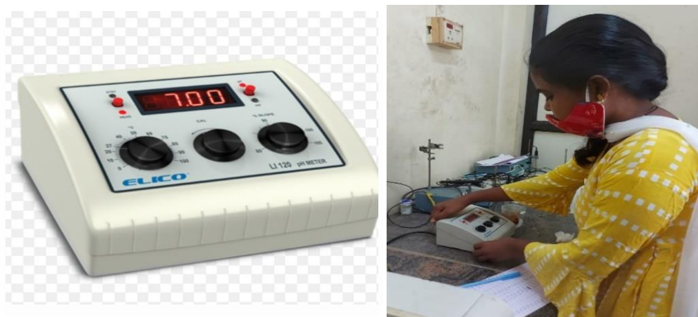
Plate 3.4 Determination of pH using pH meter
