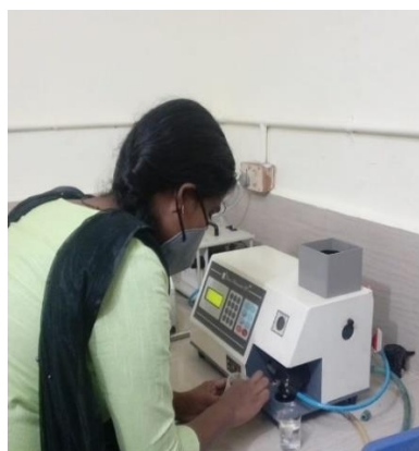
Plate 3.8 Determination of potassium by using Flame Photometer
