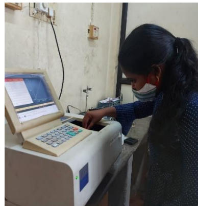
Plate 3.7 Determination of phosphorous by using UV Spectrophotometer
