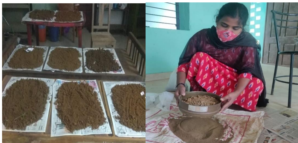
Plate 3.2 Sieving of air- dried soil samples with 2 mm sieve
