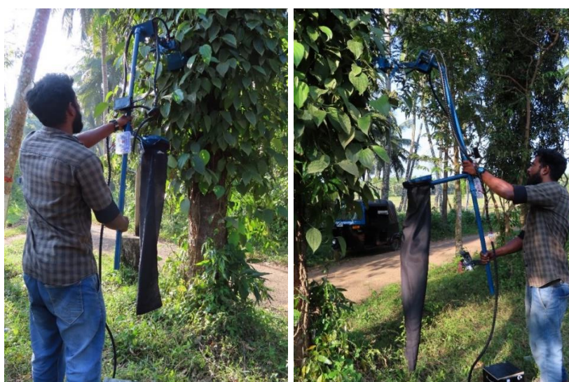
Plate 4.7 Performance evaluation of robotic black pepper harvesting system
