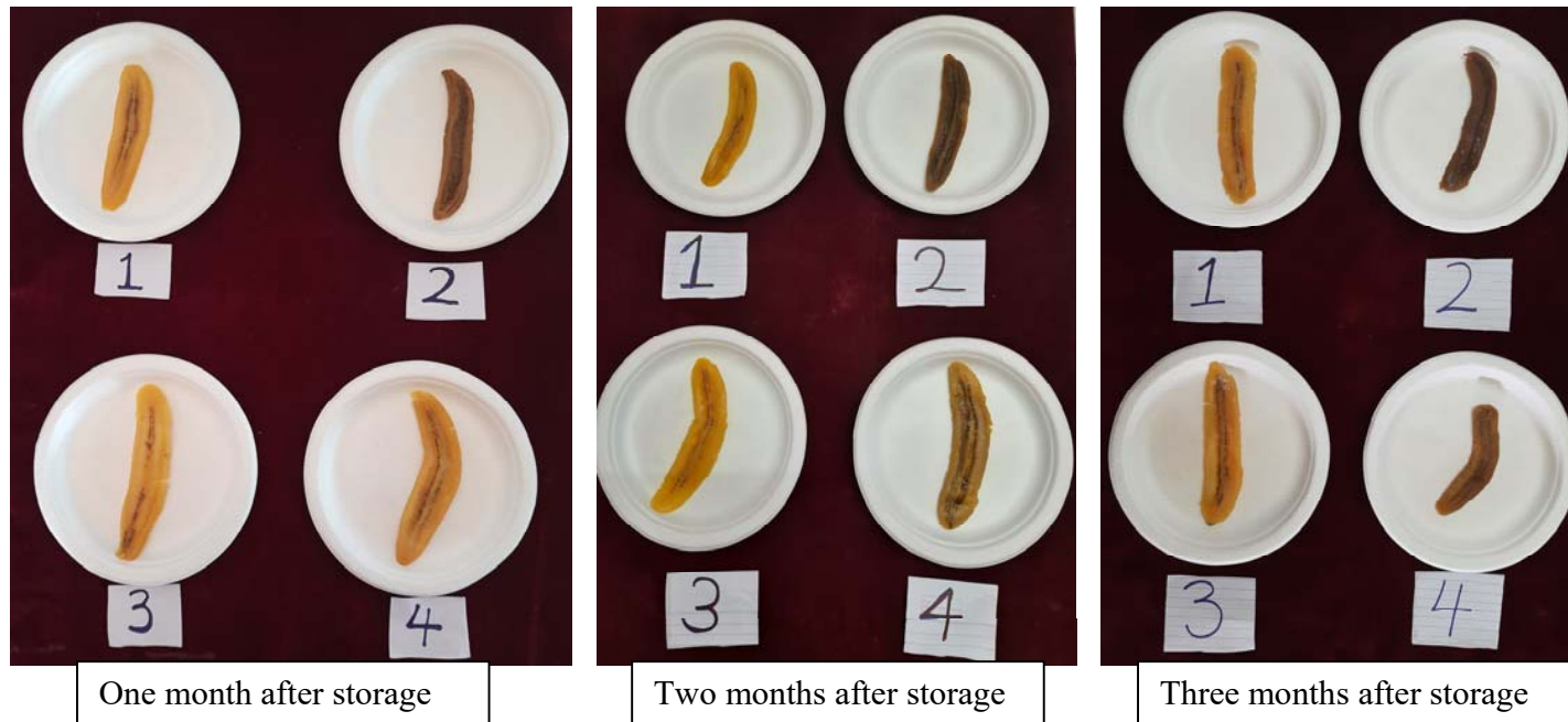
Plate 16. Storage changes in vacuum packaged intermediate moisture bananas [1= polyethylene laminated aluminium pouches+ ambient temperature, 2= LDPE (200 gauge)+ ambient temperature, 3= polyethylene laminated aluminium pouches+low temperature, 4=LDPE (200 gauge)+low temperature]
