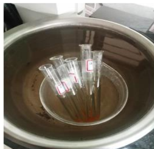
Tubes were heated at 95°C for 10 minutes and absorbance was measured at 540 nm
