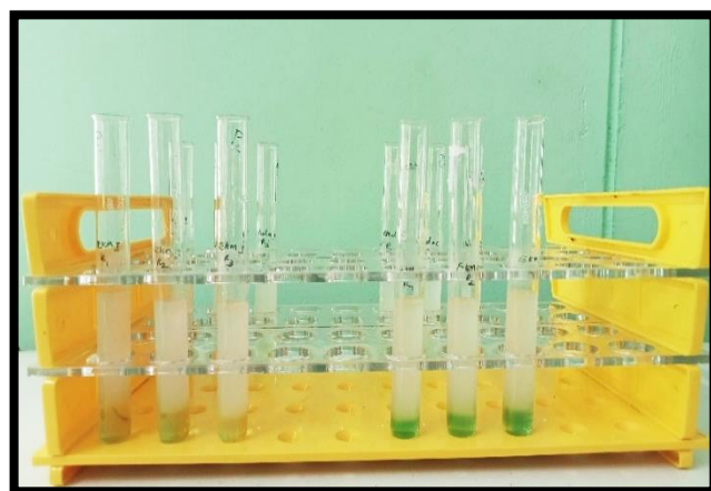
iv) After heating intensity of green colour denotes the trehalose content
