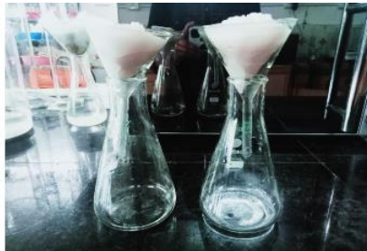
The filtrate with a gelatinous white material was separated using whatman no. 1 filter paper
