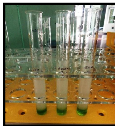
iv) After heating intensity of green colour denotes the trehalose content
