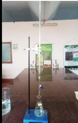
ii) Titrating contents of each flask with 0.05 N NaOH until the appearance of blue colour
