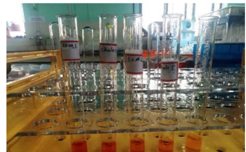
Tubes were heated at 95°C for 10 minutes and absorbance was measured at 540 nm
