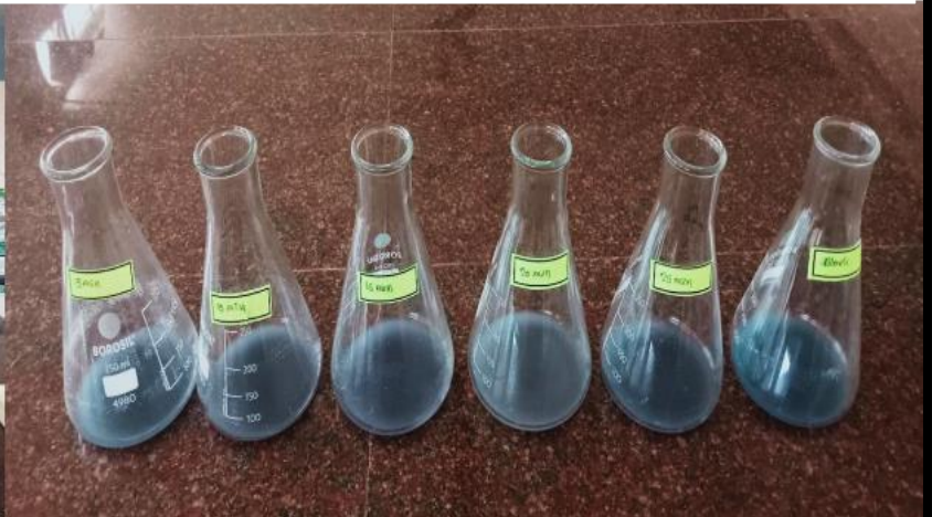
ii) Titrating contents of each flask with 0.05 N NaOH until the appearance of blue colour
