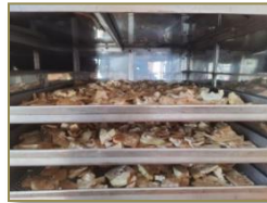
Dried in cabinet drier at 55 – 60 0 C for 8 -12 hours
