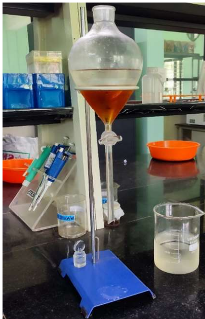
Plate 3. Extraction of solvent phase using separatory funnel
