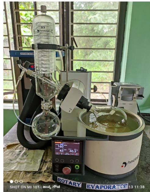
Plate 4. Vacuum rotary evaporator
