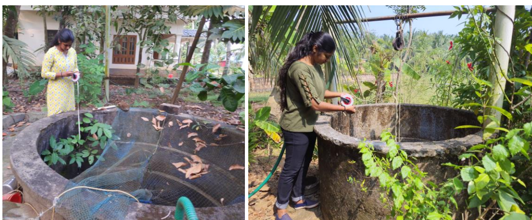
Plate 3.2 View of taking the water table level
