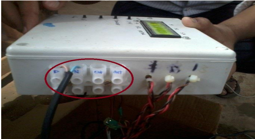
Plate 3.7 AC (230 Volts) input and output connecting terminals
