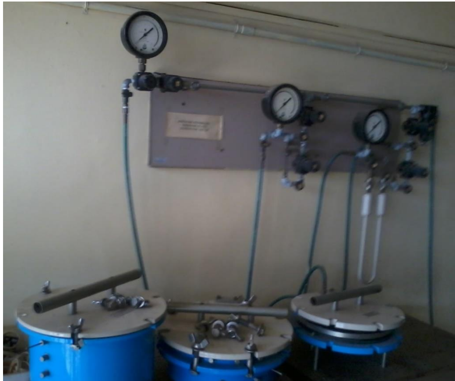
Plate 3.4 Pressure plate and membrane apparatus
