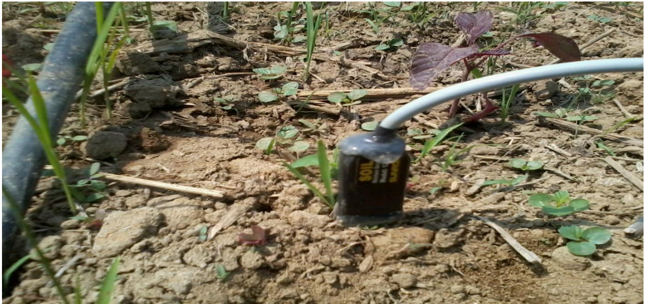
Plate 4.2 Field evaluation capacitor sensor in amaranthus crop
