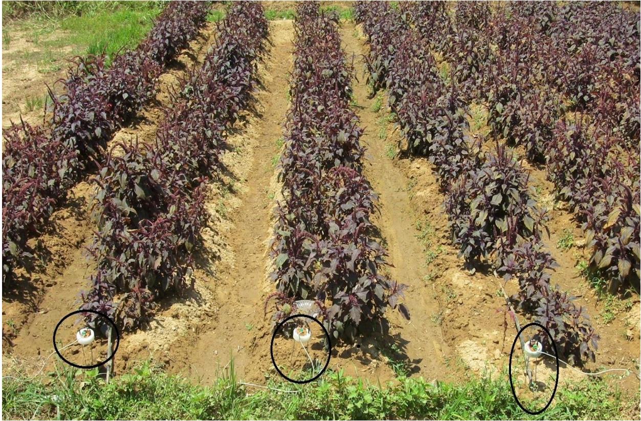
Plate 4.1 Field evaluation electrical conductivity sensors in amaranthus crop
