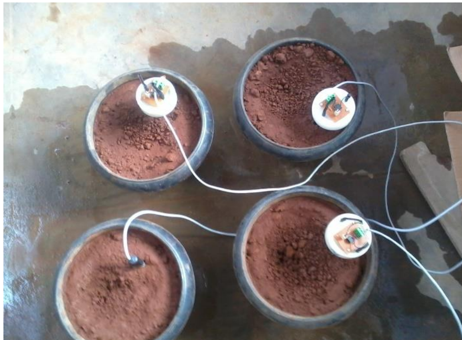
Plate 3.5 Calibration of soil moisture sensors in different soils
