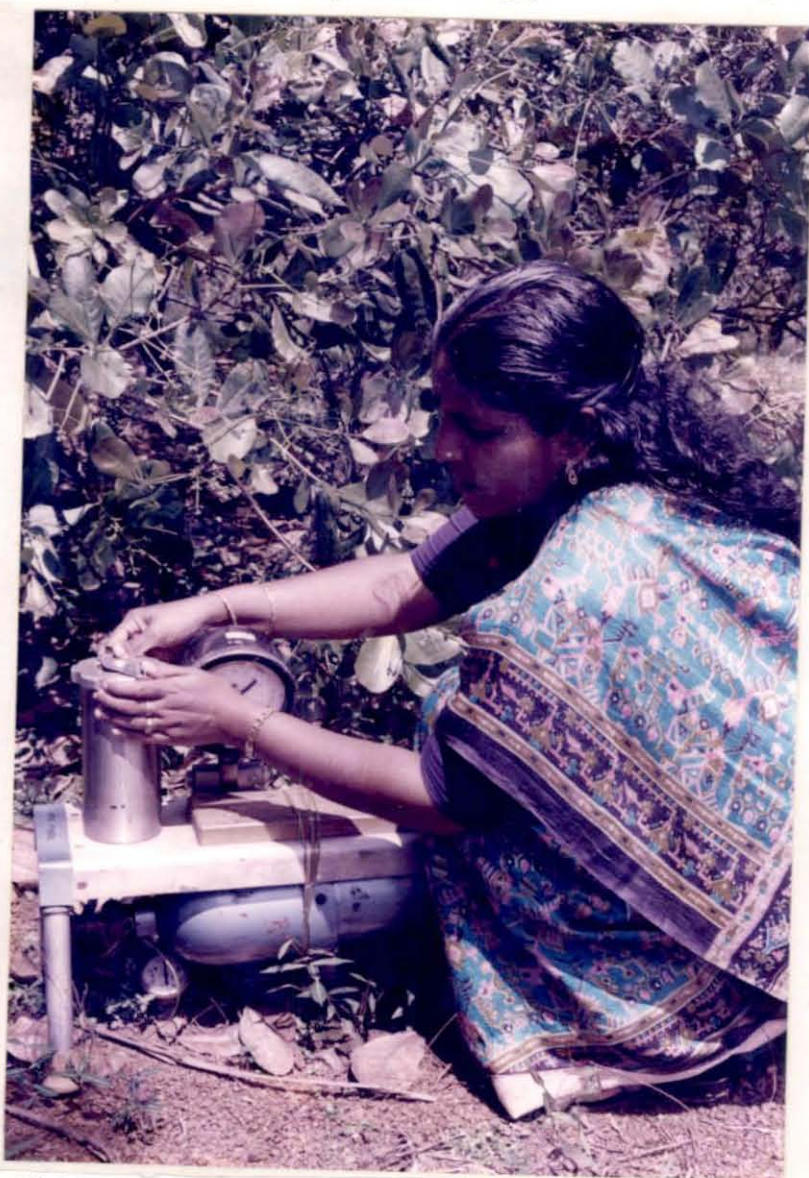
Plate 2. Field measurement of leaf water potential using Scholander type pressure bomb
