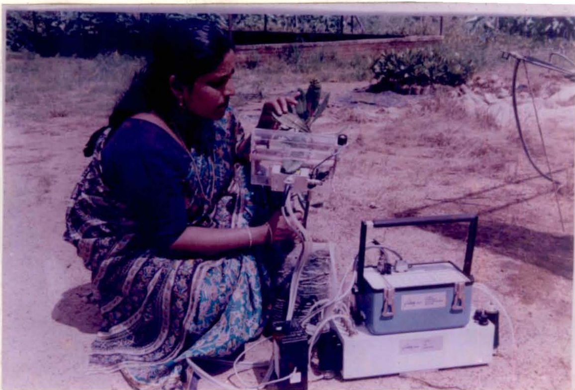
Plate 1. Field measurement of net photosynthesis, transpiration rate, stomatal conductance and leaf temperature using portable infrared gas analyser
