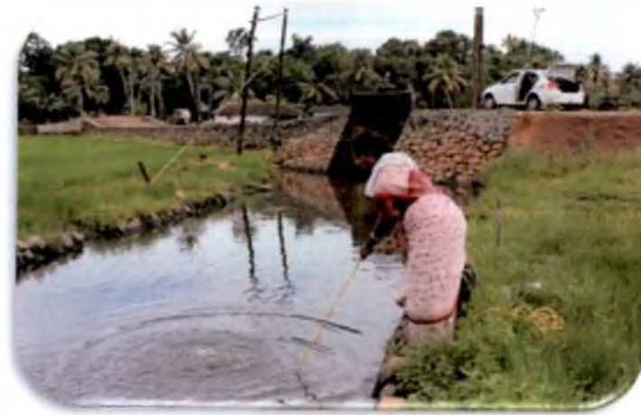
Plate 4. Collecting sediment samples from canals using Van- Veen Grab
