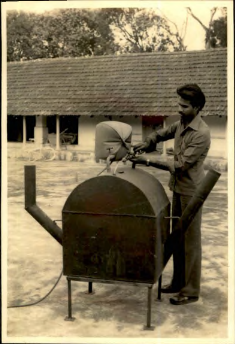
Plate VI Modified pilot plant New K.A.U. model with recirculation of bio-gas
