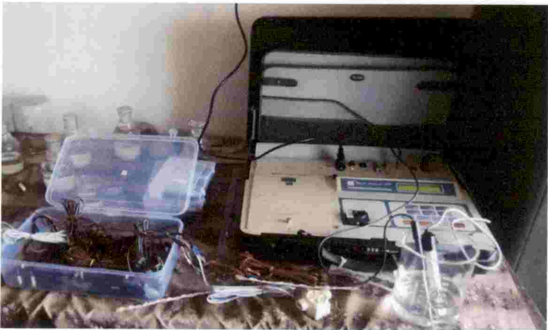
Plate 14. Electrical conductivity by EC probe in salt solution
