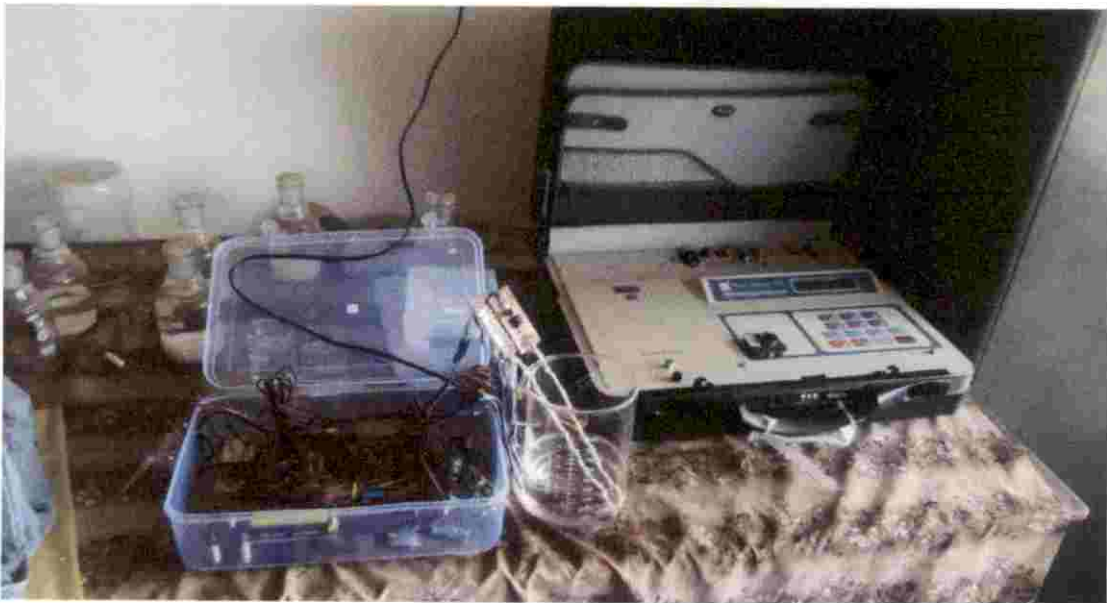
Plate 12. Calibration of capacitor type moisture sensor in salt solution
