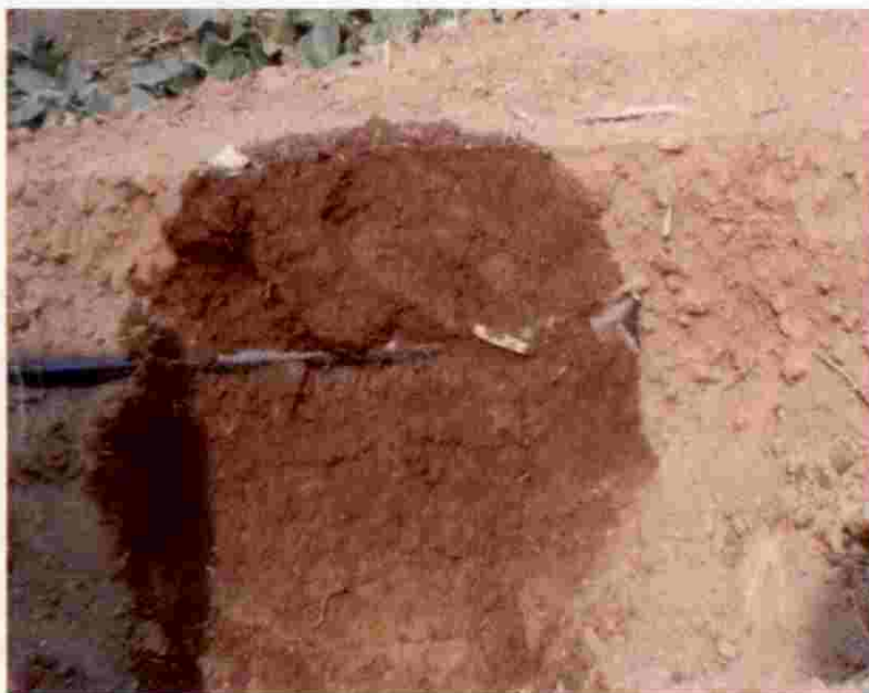
Plate 4.1 A view of vertical profile with lateral at 10 cm depth without crop
